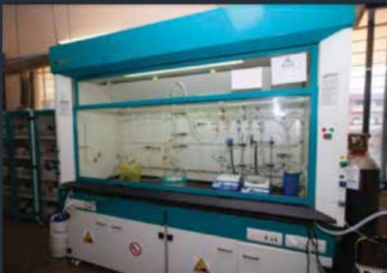
Schlenk Line Customised Perform reactions in inert atmosphere
