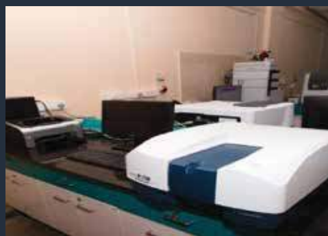
UV-Vis-NIR Spectrometer JASCO V770 Liquids 200-3200 nm, 4 to 90 degree Celsius Solids: 200 to 2500nm
